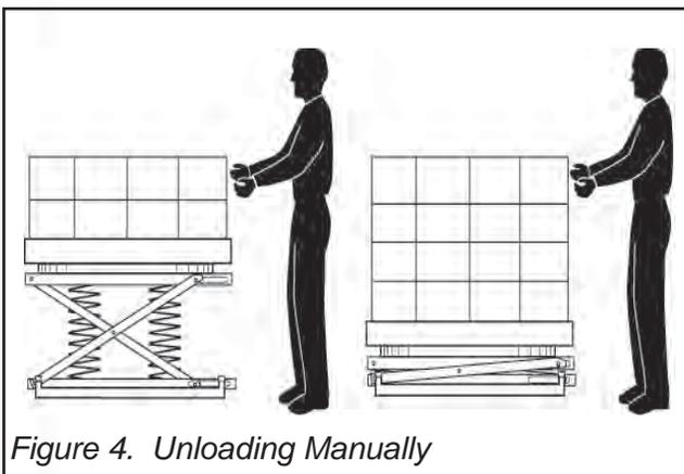
Figure 4. Unloading Manually
